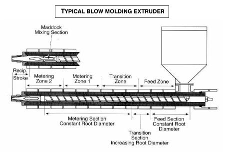
**PP-** Use a ramped profile starting at 330°F and increase the set points in steps through the extruder feed, compression, metering and head sections to a temperature set point of 370 °F.
